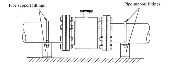
Figure 4.2 Example of Pipe Fixing Procedure
